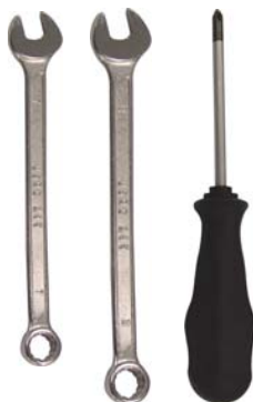
2-Use a spanner 7 mm. and 8 mm. a medium cross screwdriver.
