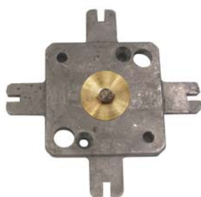
10- Install the LPG aluminium front part of the firing head cod. BFT12119 (Natural Gas cod. BFT12116) and the LPG (Natural gas) nozzle. The notch of the nozzle must be in the correct position.
