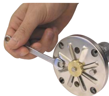
4-Remove the cables of ignition and ionization.
