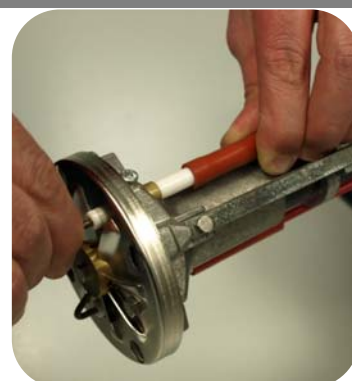
4-Remove the cables of ignition and ionization.
